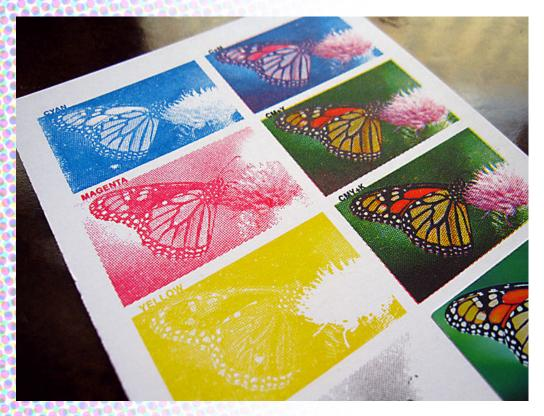
These halftone dots are varied in size and sprayed at different angles to allow the colors to mix with a wide range. This creates a pattern called a **Moire pattern** and the separated colors are called **color separations**
